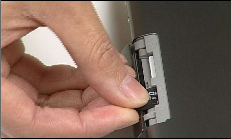
Figure 3-5. Removing Micro-SD Card
