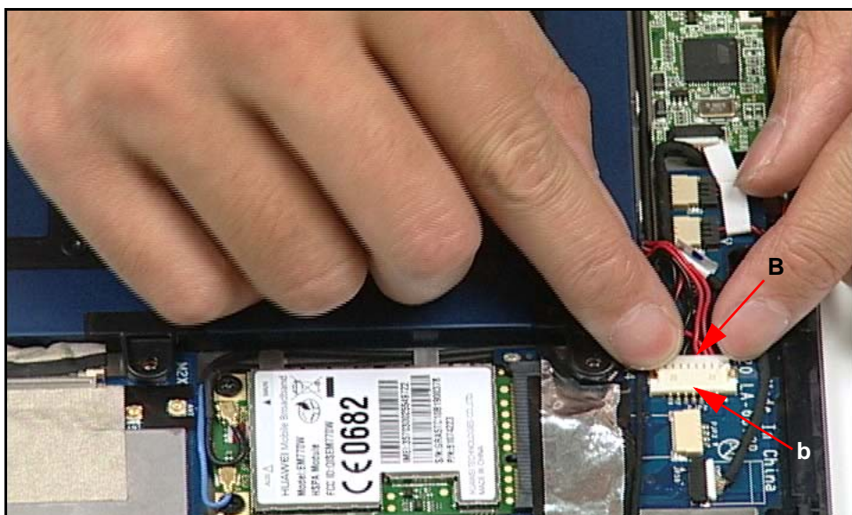
Figure 3-26. Disconnecting Battery Cable
