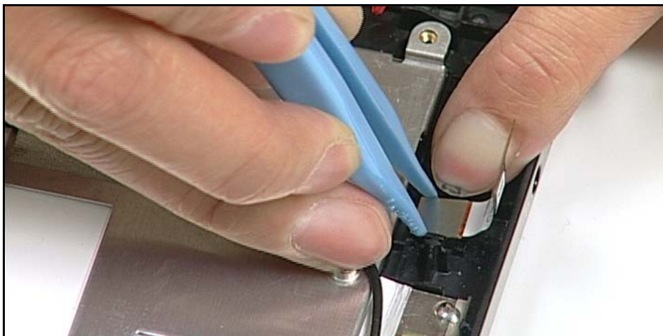
Figure 3-53. Removing Front CCD
