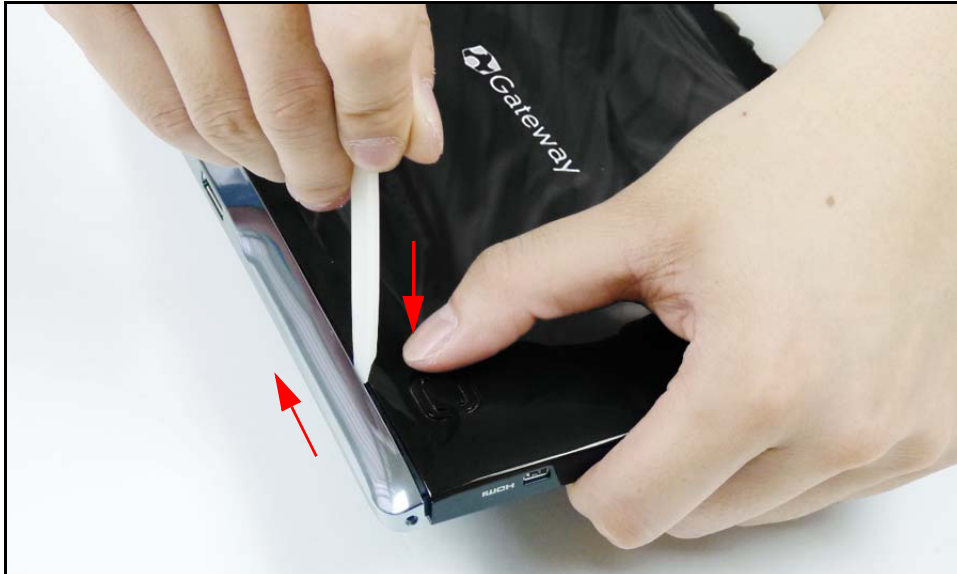
Figure 3-12. Removing the Bottom Cap (1 of 3)
