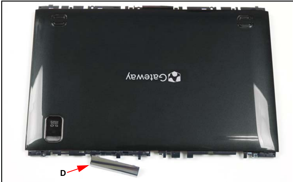
Figure 3-18. Installing the Lower Case (1 of 3)
