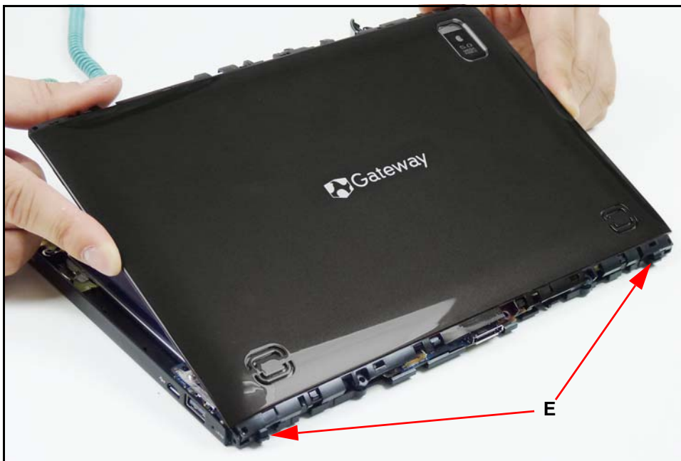
Figure 3-19. Installing the Lower Case (2 of 3)
