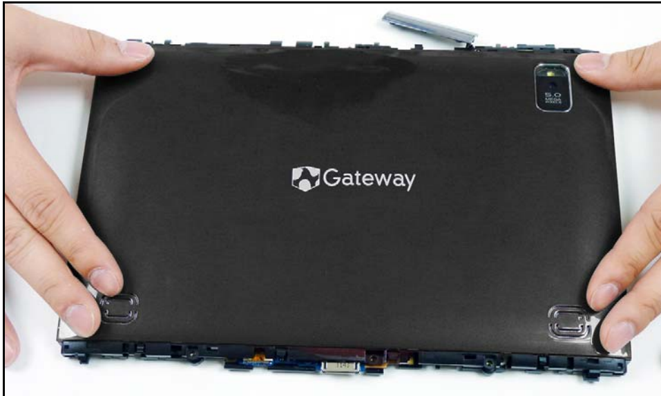
Figure 3-20. Installing the Lower Case (3 of 3)
