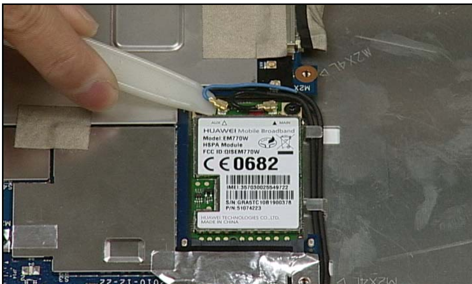
Figure 3-29. Disconnecting 3G Cables
