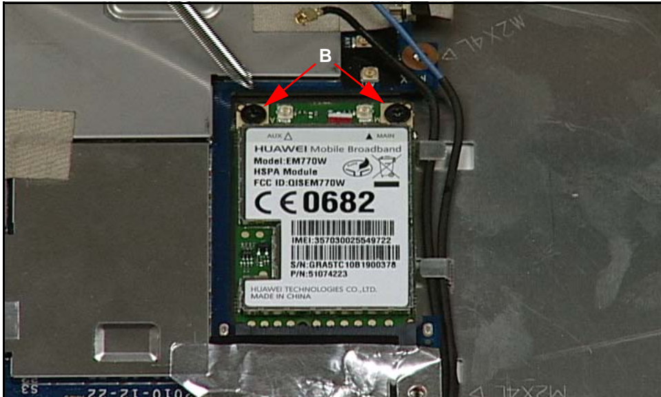
Figure 3-30. Removing 3G Module Screws
