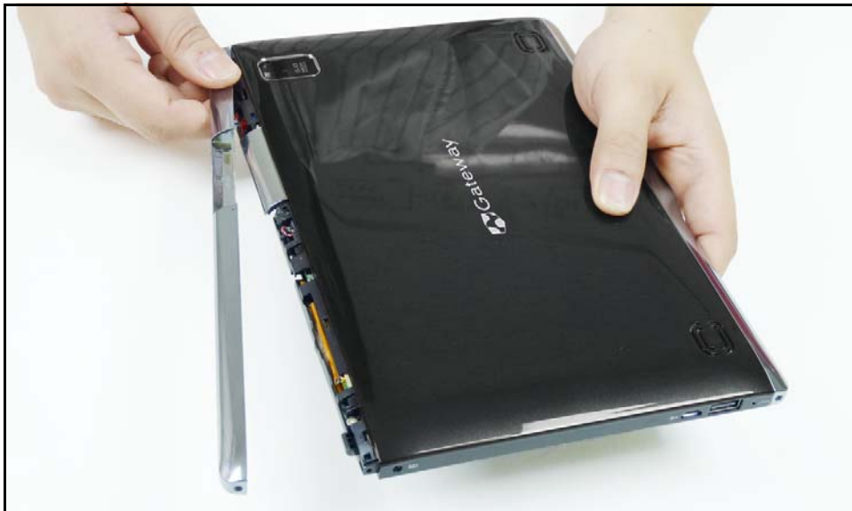
Figure 3-11. Removing Top Cap (3 of 3)
