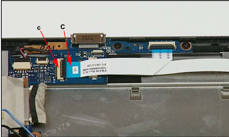
Figure 3-34. Disconnecting Docking Board FFC from Mainboard
