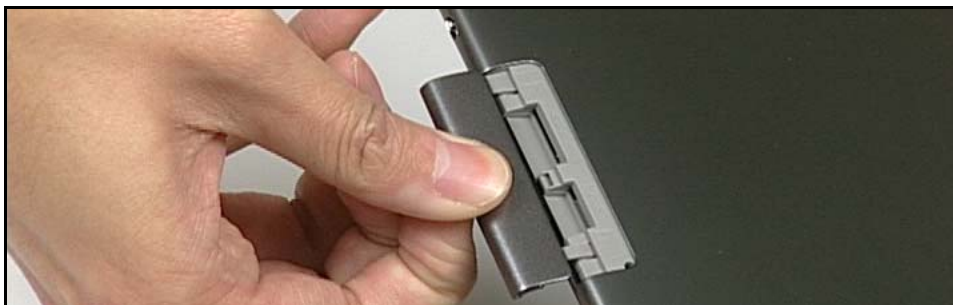
Figure 3-3. Opening SIM/Micro-SD Card Cover
