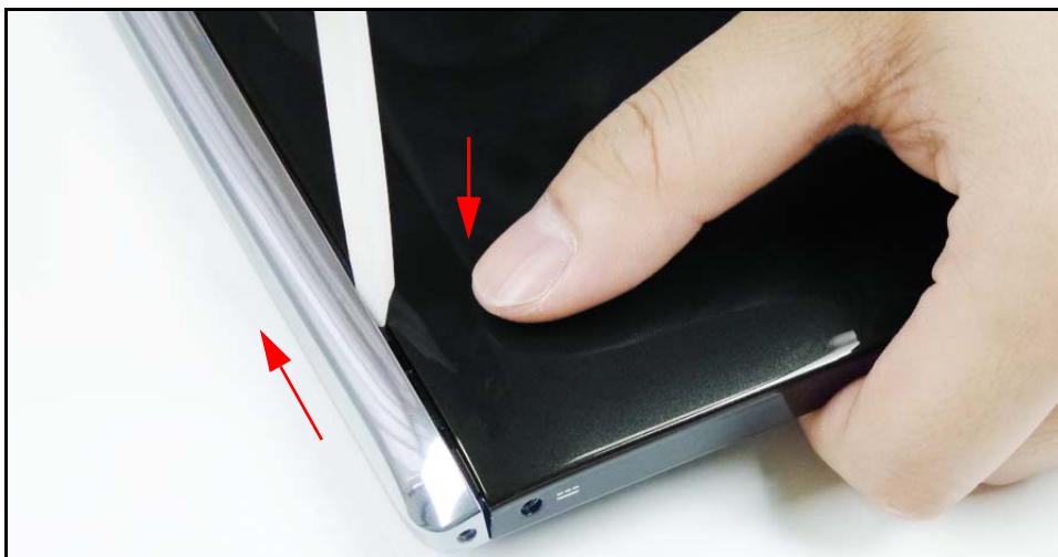
Figure 3-9. Removing the Top Cap (1 of 3)
