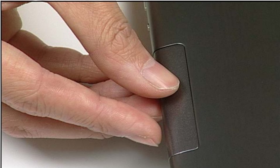
Figure 3-6. Securing SIM/Micro-SD Card Cover
