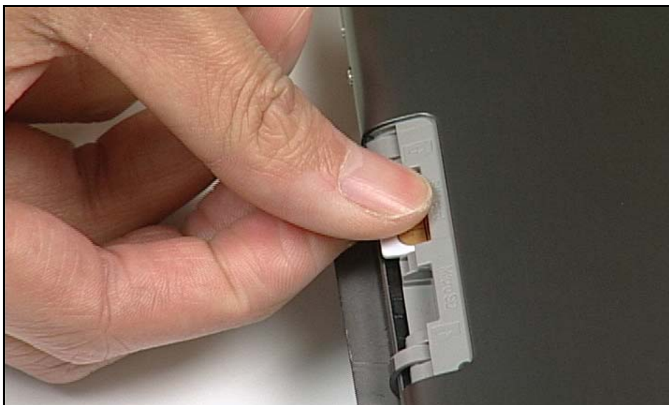
Figure 3-4. Removing SIM Card
