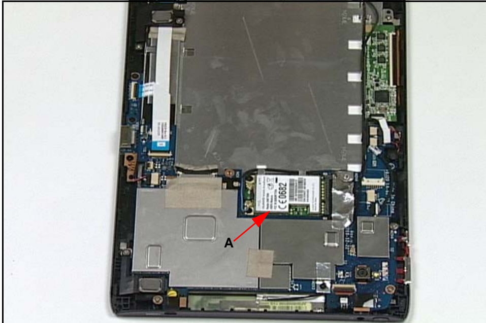
Figure 3-28. 3G Module on LCD Support Plate
