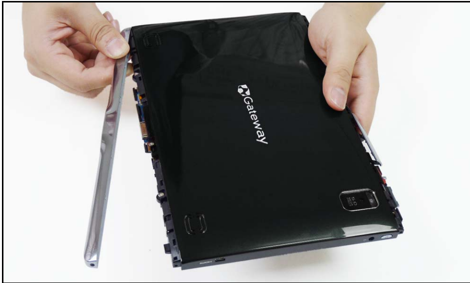
Figure 3-14. Removing the Bottom Cap (3 of 3)
