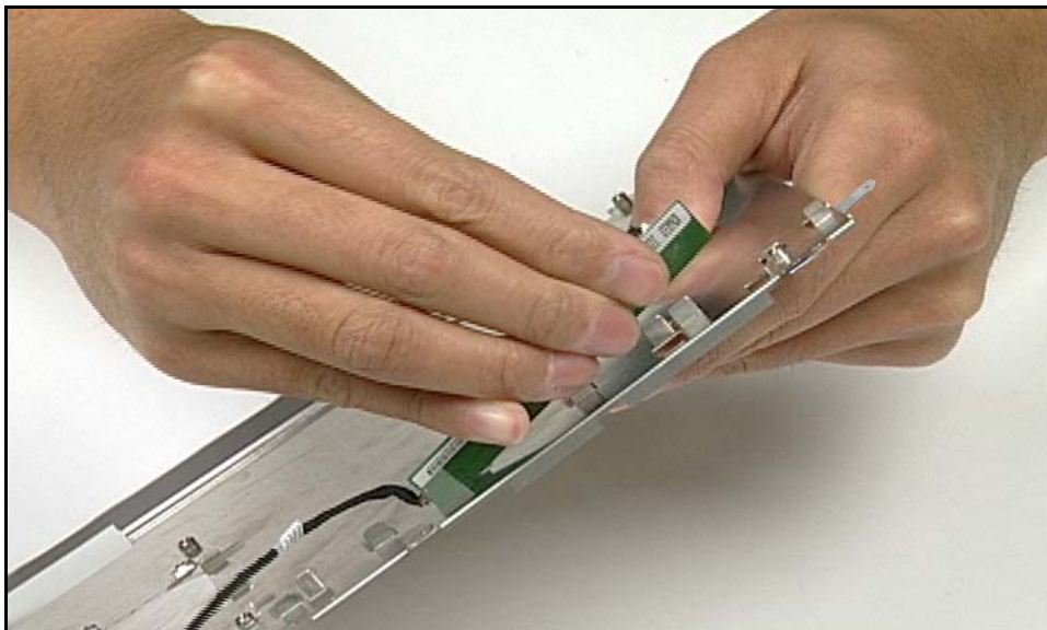
Figure 3-69. Removing Control Board (2 of 2)
