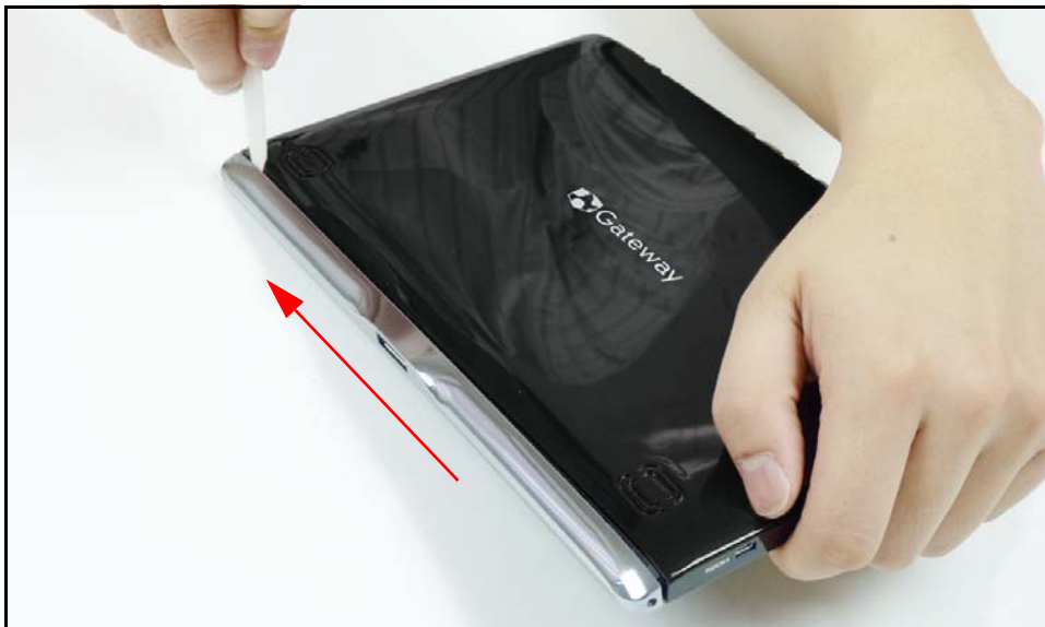
Figure 3-13. Removing the Bottom Cap (2 of 3)
