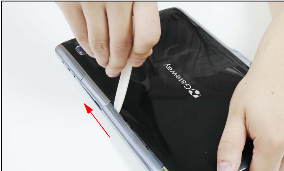
Figure 3-10. Removing the Top Cap (2 of 3)
